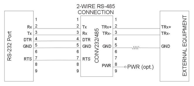
FIGURE 1, CONNECTION DIAGRAM
