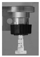
To set the downtilt angle exactly you must look horizontally at the scale. The lower edge of the gear wheel must be used for alignment purposes.
