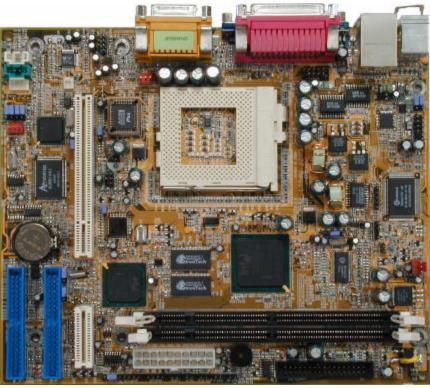
expansion cards for these functions. The G370IF10 is ideal for kiosks, instrumentation, and other applications where a powerful but compact PC platform is required. Optionally available riser cards may be added to enable two PCI expansion cards, or one PCI card and one AMR card, to be added to the systems and still maintain a low profile.
