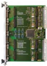
A set of 16-position rotary switches allows easy configuration of VME Short I/O and Memory addresses. Interrupt routing from the IP slots to the VME IRQ's can be done in two ways: programmable by software or selection of predefined sets by a rotary switch.
