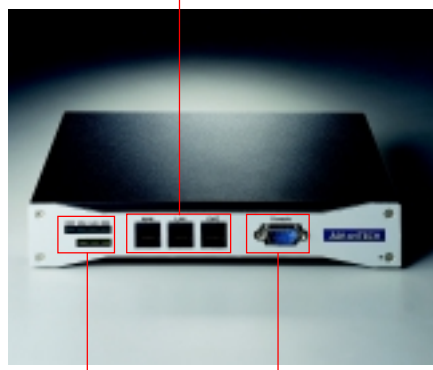
7 LED indicators (Power x1, LAN x6) RS-232 Console port
