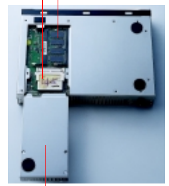
Removable cover allows easy maintenance and software upgrades
