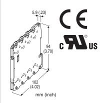
Operating temperature: -20 to +55°C (-4 to +131°F) Operating humidity: 30 to 90 %RH (non-condensing) Mounting: Installation Base (model: M6SBS) Weight: 60 g (2.1 oz)
