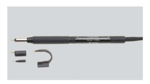
The 1205 RF Probe 20 dB is a passive 10:1 RF voltage probe with a built in 50 V DC block. It has been designed to allow users of RF test equipment to use standard signal tracing techniques. The probe makes it possible to conveniently and accurately monitor or inject signals up to 4 GHz into RF circuits without significantly loading or detuning them.
