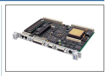
Resolutions of 800 x 600 256-color and 1,024 x 768 16-color in interlaced and noninterlaced modes are supported.
