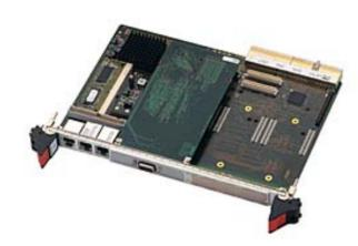
The D3 is a single-board computer for embedded applications based on the Kahlua II PowerPC. It can be used in a CompactPCI system slot or as a stand-alone card.
