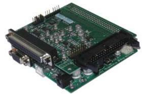
Since the dspstak I/O module is separate from the DSP module, custom interfaces can be created quickly and inexpensively.
