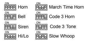
Note: The code-3 Horn and Tone alert sounds are reserved for emergency evacuation signaling. They should not be used for any other purpose!
