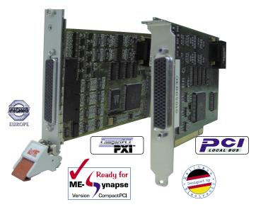
Versatile analog output board at a reasonable price: This solid standard D/A board gives you up to 16 voltage outputs with 12 bit resolution. On the model "UI" you can also use 8 of the lines for current output, if required. The current ranges are 0...20 mA and 4...20 mA.
