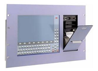
A Human-Machine Interface (HMI) is a computer which handles the communication between machines and humans. Thus it deals with any aspects that have an impact on a user's interaction with that system. A machine can be anything from a wristwatch to a large factory. The communication can be the human pushing a button or the machine flashing a lamp.
