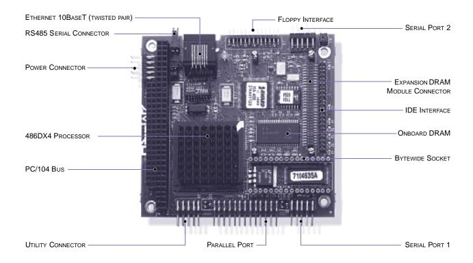
The CoreModule/4GE, along with the CoreModule/4GV, is the first of Ampro's new family of high integration PC/104 CPUs. These modules pack 486 processing power together with all standard embedded PC product features—including CPU and memory subsystems, communications ports and disk interfaces—plus key additional features into less than 14 square inches of board space. This high level of integration allows a single module to serve a wide range of embedded applications.
