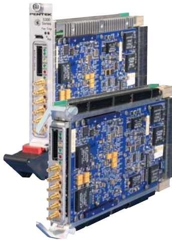
Model 53620 COTS (left) and rugged version
