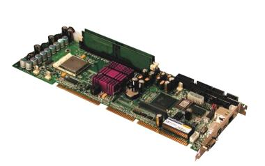
Our VTC5611 Intel® Pentium® 4 processor-based PICMG® PCI/ISA compliant passive backplane single board computer addresses wide ranging, high performance, long-life applied computing applications.
