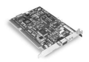
The SST Profibus ISA card connects your ISA bus computer to Profibus DP, FMS client\*, FDL and the S7 Communication Port.
