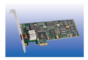
Offering E1, T1, or ISDN PRI digital network interfaces, the Diva PRI/E1/T1-CTI provides proven connectivity with a wide range of PBX and switch systems. Because of its comprehensive implementation of signaling protocols, including all international ISDN variants and QSIG, the Diva PRI/E1/T1-CTI also enables many sophisticated supplementary services, which can then be used by computer telephony integration applications.
