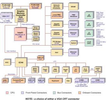
NOTE:- a choice of either a VGA CRT connector or a 2nd COM port is available for the Front Panel
