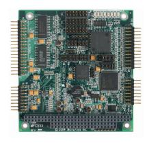
The MPC555 Analog and Digital I/O module provides 16 channels of analog input to PC/104 systems that run high or low speed CPUs. The module also includes 24 bits of digital I/O, 4 general-purpose input jumpers, 8 user LEDs, and three general-purpose counter/timers. Additionally, up to 8 channels of analog output are available.
