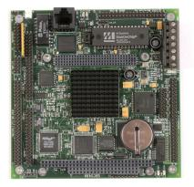
The SBC0489 packs a fast 486DX processor with a large amount of industrial I/O in a 5" x 5" format. It offers plenty of memory capacity, and copious amounts of storage. In addition to the core processor and memory, an ample mix of serial, parallel, EIDE, floppy, keyboard, mouse, VGA, touchscreen, Ethernet, digital I/O, and analog I/O provides a single board solution to many design challenges.
