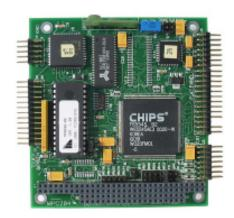
The MPC204 is a low cost PC/104 operator interface solution. It allows flat panel LCD displays to be driven with standard PC code. The VGA subsystem supports monochrome and active matrix color. Standard VGA CRT monitors can also be driven. Panel and screen resolutions from 320x200 to 1280x1024 are supported.
