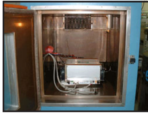
ACT/Technico Temperature Cycle Chamber
