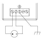
Connect an appropriate source of 24VDC to the power supply. Terminals accommodate one AWG #14 (avg. 2.1mm<sup>2</sup> cross section) to AWG #22 (avg. 0.36mm<sup>2</sup> cross section) wire, or two wires up to AWG #18 (avg. 0.86mm<sup>2</sup> cross section). Use copper wire rated for 90 degrees C. When inserting two wires in the same position, the wires must be the same size and type (solid or stranded).
