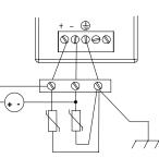
For agency compliance, external MOV suppression is required from both the positive and negative input to frame ground or at the power line input of a system enclosure.
