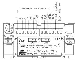
**Note:** The model DT700000 will NOT have a screw terminal installed at Terminal 2 (V+), since it is NOT required for operation, and is not internally connected. The DT700M00 uses the V+ screw terminal to mount the MLPS power supply. It is not internally connected to the unit.
