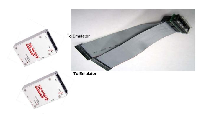
Please Note: The E8U-40CBL Adapter is designed for 40 pin target DIP sockets. Our emulators receive power or detect power from PIN 32 of the DIP connector. It will download two of 8-bit data from two EeRom-8U through the 32-pin cables to 40-pin DIP target.
