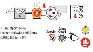
2. Slowly turn the setpoint screw clockwise until the Status OPEN LED just turns ON.
