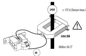
DANGER: 5A CTs can present hazardous voltages. Install CTs in accordance with manufacturer's instructions. Terminate the CT secondary before applying current.
