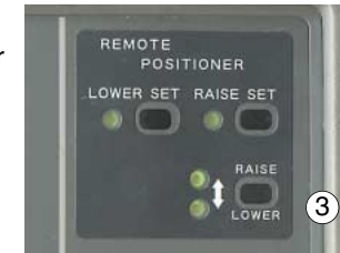
3:Remote boom positioner switch
