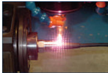
Laser welding fuses metal parts together without excessive heat, which could be damaging to internal electronics
