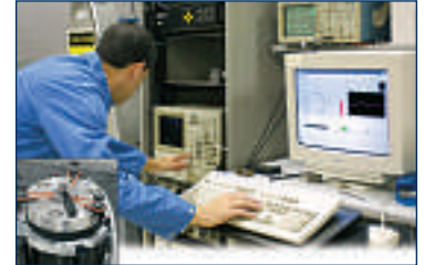
Primary Accelerometer Calibration Accelerometer is mounted to an air-bearing shaker beneath a laser vibrometer
