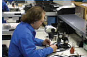
Precision sensor assembly under microscope
