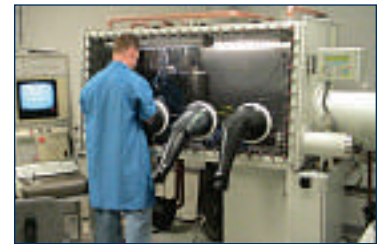
Glove box handling with laser welding permits inert gas to be added within the sensor
