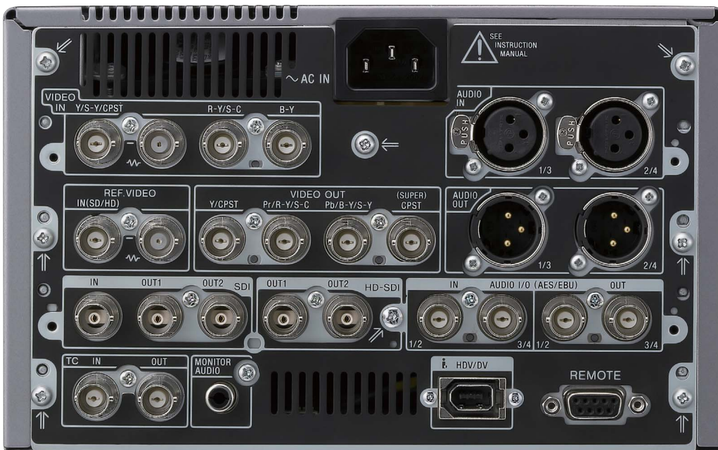
Rear panel of the HVR-1500 (with the optional HVBK-1505 board)
