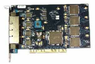
Consolidate multiple server 10/100 Mbps ports onto a single low cost network interface card (NIC).
