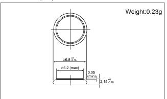
**Note:** This bare cell diagram is for size reference only. Please refer to the tab configurations at the end of this section for available tabs.
