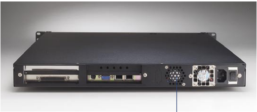
One 10-CFM cooling fan is on rear-end
