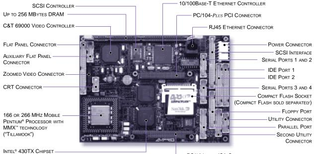
The Little Board/P5*x* raises the bar for Pentium-based embedded-PC designs. The latest laptop chipsets are combined with a rugged, robust design to provide a highly reliable single-board solution for embedded applications that demand small size, low power consumption, and high functionality.
