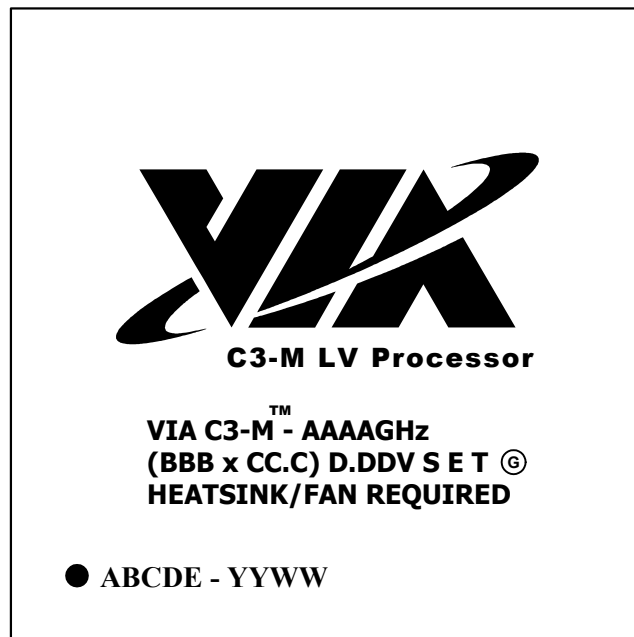
Figure 5-4. C3-M LV Top Marking Diagram
