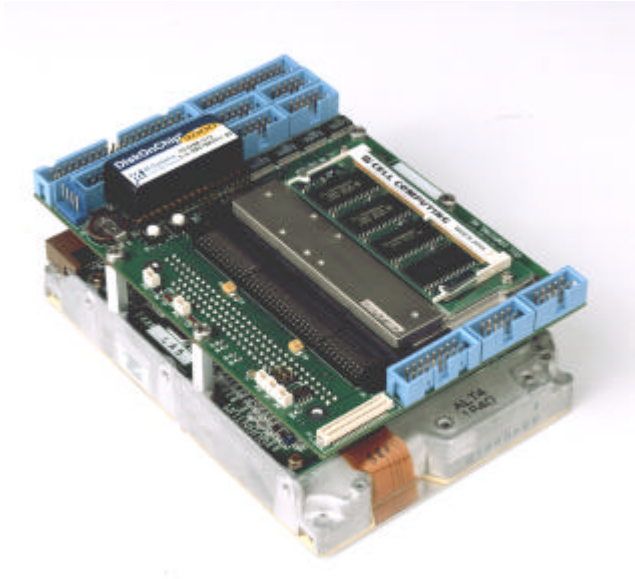
The Mighty Mite configured with 233MHz Pentium CardPC (3.5" disk drive not included)
