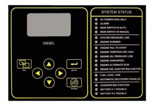
**Description** – Firetrol® combined automatic and manual Mark IIXG based diesel engine fire pump controllers are intended for starting and monitoring fire pump diesel engines. They are suitable for use with both mechanical and electronic type engines. The controller is available for 12 or 24 volt negative ground systems, using lead acid or Nickel-Cadmium batteries. The controller monitors. displays and records fire pump system information.
