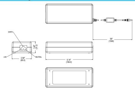
1.47" (H) x 2.56" (W) x 6.14" (L) 37.2 mm (H) x 65.0 mm (W) x 156.0 mm (L) AC Input Connector: IEC320, C6 AC Input power cord sold separately
