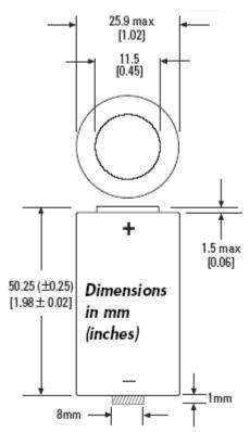
1mm of clearance must be allowed at this point between negative end cap and any adjacent surface.
