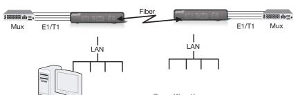
MediaBand-4 transports up to four E1/T1 circuits across a wide variety of fiber links. The same fiber can be used to simultaneously transport Ethernet services.
