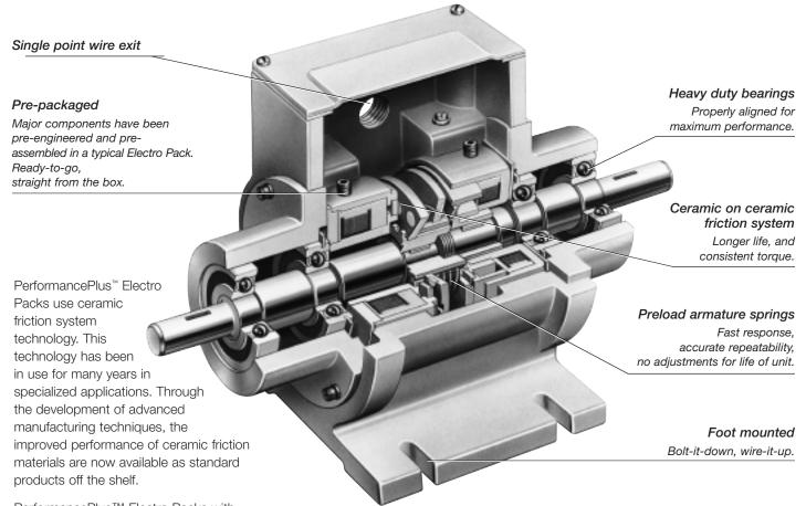
PerformancePlus™ Electro Packs with ceramic friction material are rugged, preassembled clutch and brake combinations in base mounted housings. They have been designed to be installed in standard power transmission systems with V-belts and pulleys, chain and sprockets, in line couplings, and timing belt drives.
