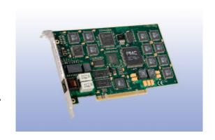
server applications. Because of its additional eight dedicated DSP-based media processing resources, up to eight calls out of the total E1 or T1 span can concurrently handle demanding operations such as V.90 data modem, high-speed 33.6 kbps fax, or enhanced echo cancellation.
