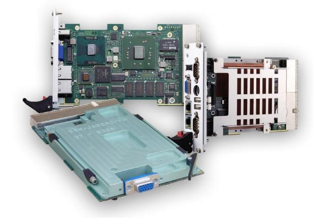
▶ Performance/Dissipation matching your application Performance 64-bit Dual Core Intel® Core™2 Duo processor 1.5 GHz with SSE3 Best Performance/Dissipation compromise Intel® Core™ Duo processor 1.2 GHz Low Power Consumption Intel® Celeron® M 1.07 GHz
