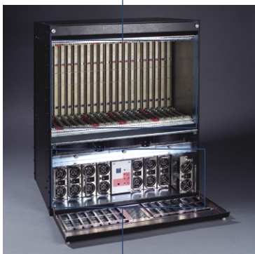
AC or DC ATX 1960 W+280 W redundant (7+1) power supplies
