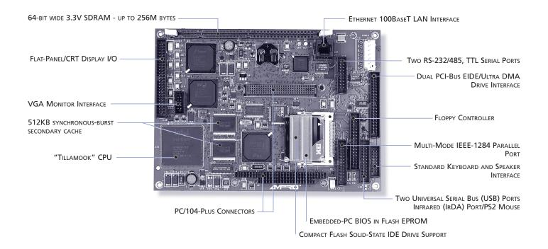
The highly integrated Little Board/P5v EBX-compatible single board computer features a powerful, low-power 266 MHz Mobile Pentium processor, advanced networking and high performance graphics. The Little Board/P5v is ideal for high volume, ruggedized, cost-conscious embedded designs that need to optimize cost vs. performance vs. power/heat requirements.
