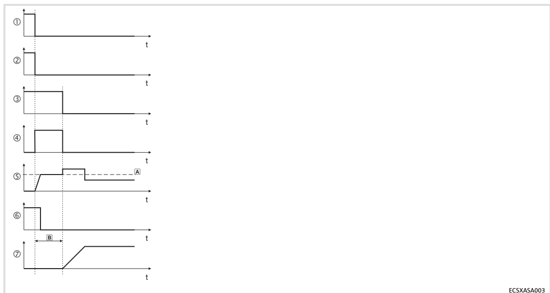
Fig.11-37 Signal characteristic - opening of holding brake
