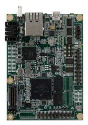
The SBC5651 is for use in small, low-power handheld and portable devices typical to medical, gaming, ticketing, and test and measurement applications. With the Freescale i.MX515 ARM Cortex-A8 multimedia processor at its core, the SBC5651 can consume as little as 1W with user-programmable speeds up to 800MHz. The SBC5651 can be powered through the USB OTG connector, a standard terminal block, StackableUSB, or single cell Lithium lon battery.
