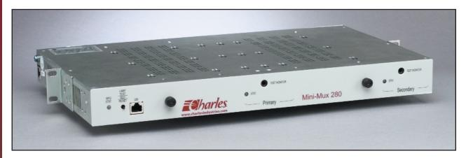
Charles Industries' Mini-Mux 210 (E1 version) and 280 (T1 version) are industry leading M13 multiplexer solutions. The Mini-Mux 210 multiplexes E1s into a T3, STS-1, or AU3 signal. Likewise, the Mini-Mux 280 multiplexes T1s into a T3 or STS-1. Both units feature low power consumption and a small 1 rack unit footprint ideal for co-location applications.
