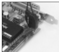
Dully gold-plated surface is reliably detected.
