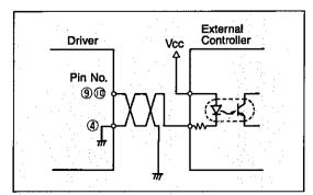
At 24V or less, a current of 10mA or less can be switched on and off at Vcc. This connection is necessary only if the speed monitor and alarm functions are used.
