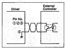
Use with a saturation voltage (voltage when power is turned on) of 0.5V or less.
