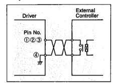
Uses a small contact point-type relay capable of switching DC 5V, 10mA.
